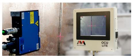
The new, all-digital MetaView combines a laser-camera sensor head with a colour touchscreen video monitor.
