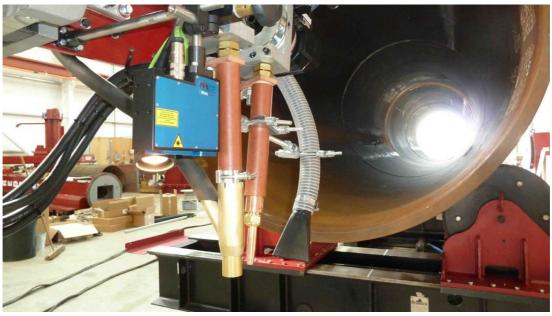
The MetaView sensor mounted on a tandem SAW head.
